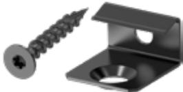
**PENETRATION DEPTH** MINIMUM deck board groove should be 1/8" tall x 1/4" deep. The material remaining below groove (dim A) must be at least 1/4". The bottom of the plastic part of the clip is not designed to contact the joist. See image to the right for a visual representation of the EDGECLIP.
